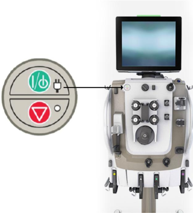
Figure Powering on the control unit
