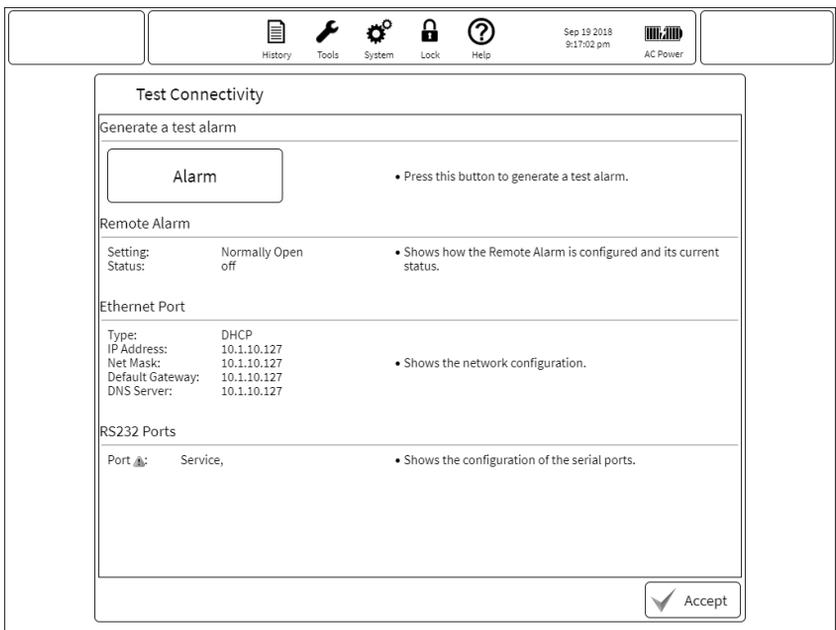
Figure Test connectivity window
