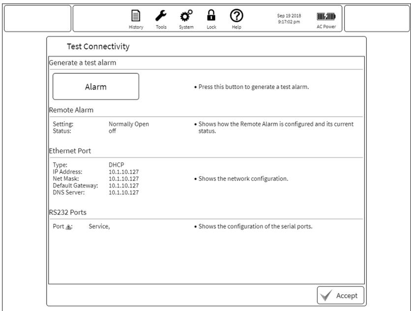
Figure Test connectivity window
