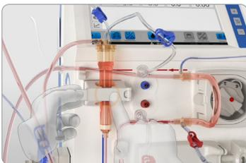
1. Press the center of the blood pump door and pull the tab to open the door.
