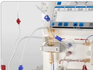
9. Attach the venous pressure transducer protector to the blue venous pressure transducer connector. Turn to secure the connections - transducer line to transducer protector and transducer protector to transducer connector on the machine.
