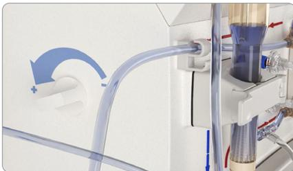
9. Once a small volume of priming fluid has reached the venous chamber, adjust the level of priming fluid in the venous drip chamber with the adjustment knob. The level should be well above the air detector head.
