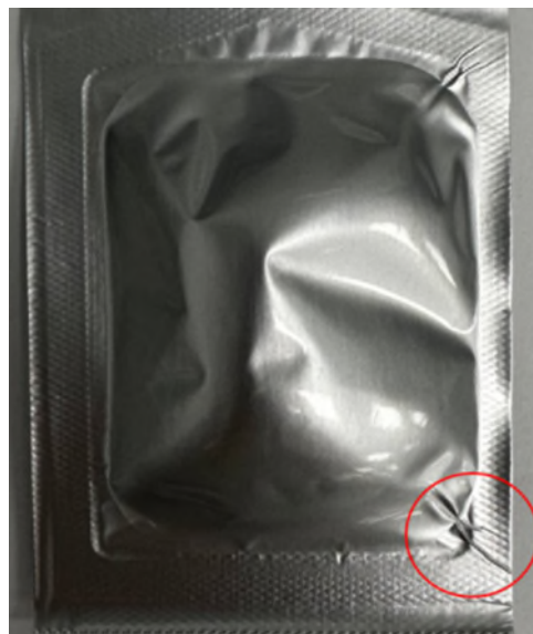
Figure 4. Weak or incomplete seal that runs to the outer edge of the packaging
